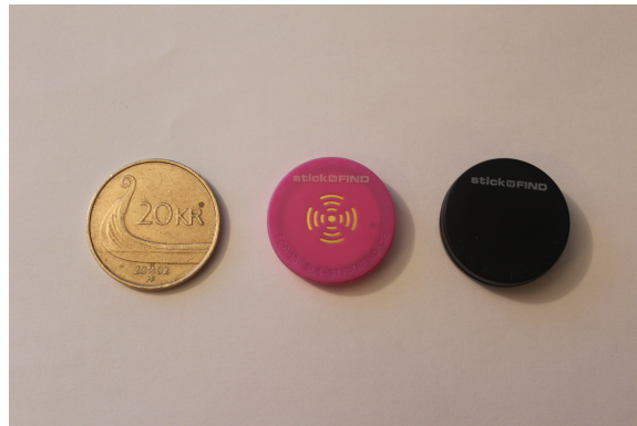
Figure 3.5: Figure showing the original StickNFind (pink) and the StickNFind Pro (black) compared to a 20 NOK coin
