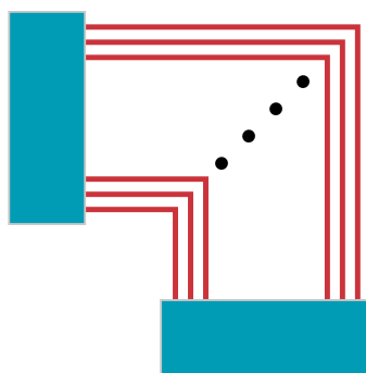
Figure 2.1: Parallel buses transfer 32 to 64 bits per clock cycle, but are prone to interference and variances in propagation delay, due to varying length of the wires.
