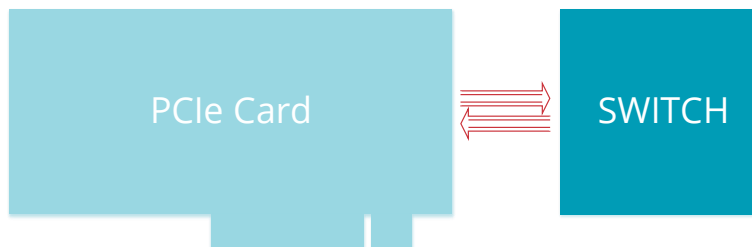
Figure 2.2: A PCIe x1 link uses four wires and transmits one bit in each direction per cycle.
