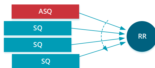
Figure 1.3: With RR arbitration, every submission queue is treated equally, including the admin queue. The controller can be configured to process a single command from each queue at a time, or in bursts.
