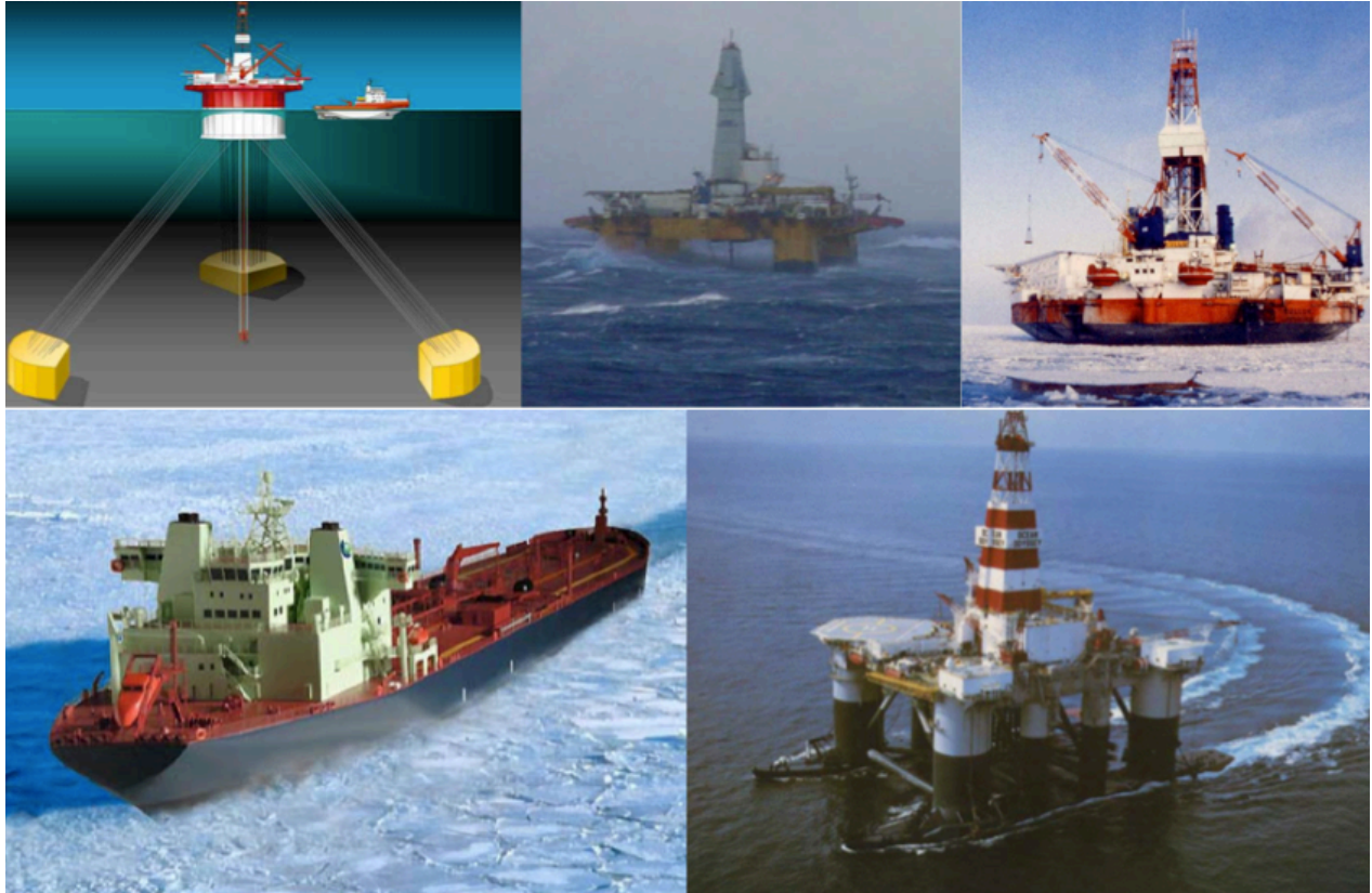
Figure 4: Winterized floating drilling structures, Arctic Semi-rigid Floater, Henry Goodrich, Kulluk, Tempera, and Ocean Odyssey (IMVPA, 2008, pp.72,77,135,107,137).
