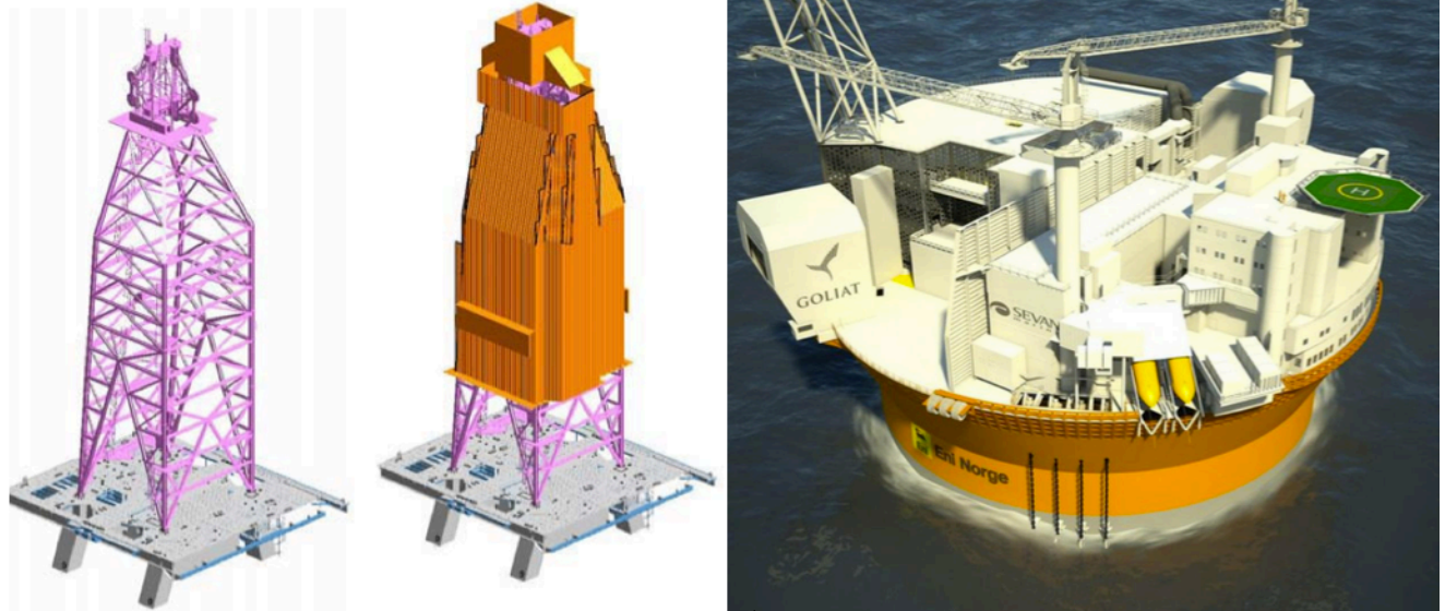
Figure 27: To the left: Derrick with and without wind shielding (Gudmestad(b), 2010). To the right: The winterized Goliat production facility (TU, 2012).
