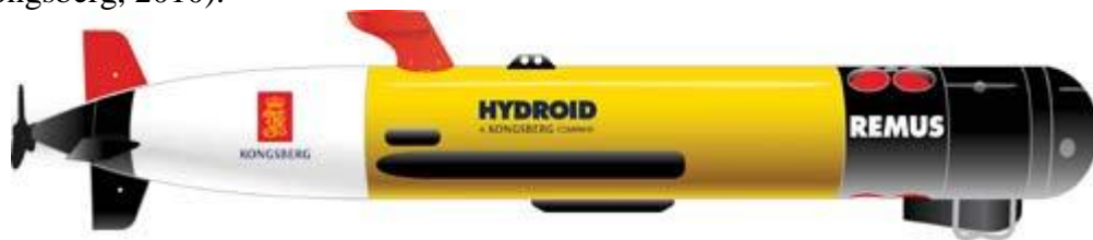
Figure 28: Autonomous underwater vehicle designed by Kongsberg and a suitable example for utilization during advanced seismic operations.
