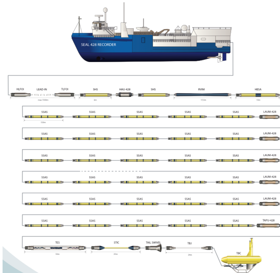
Figure 13: Example of elements and structure of a Sercel Sentinel streamer cable.
