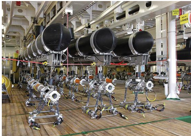
Figure 11: Seismic Source in stand by position on the gun deck.
