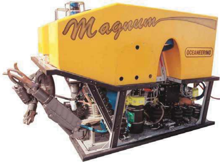
Figure 1.2: A Remotely Operated Vehicle (ROV) in support of oil and gas drilling, construction, and production activities working in ocean depths inaccessible for most human activity. Reproduced with courtesy to Oceaneering.
