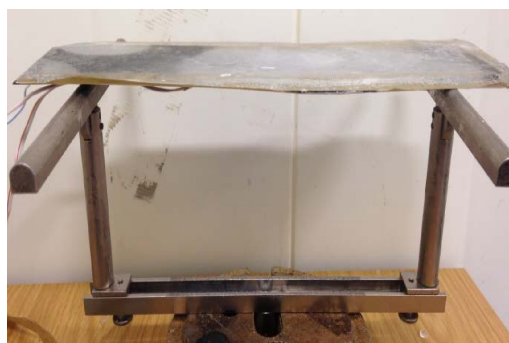
PVC and Ice sample placed for four-point bending test
