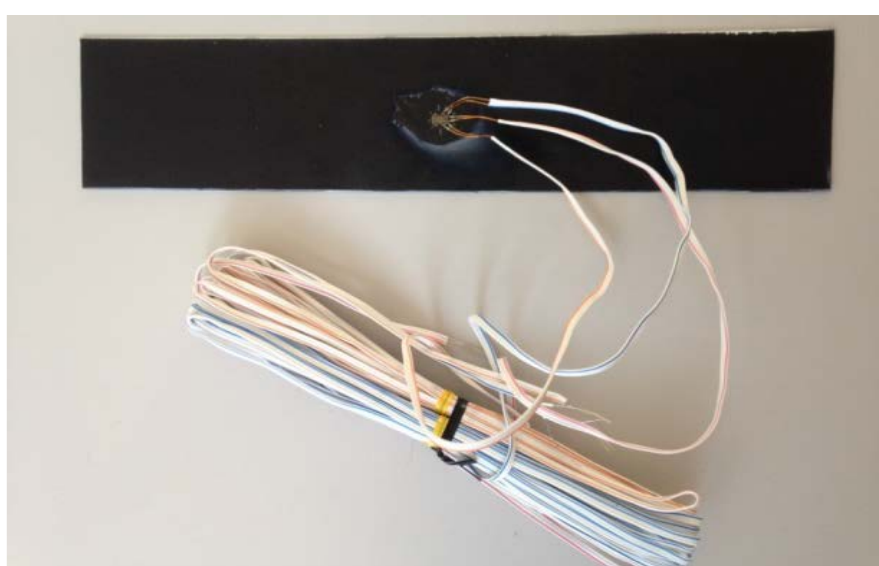
PVC Sample with Rosette Strain Gauge
