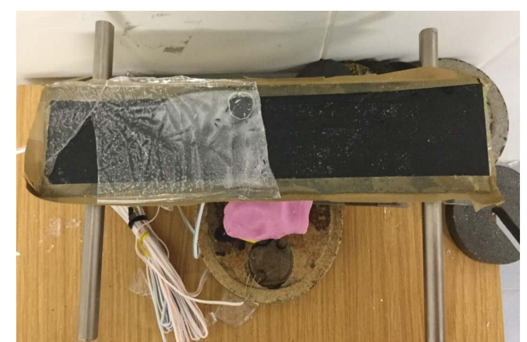
Delamination of Ice over PVC surface
