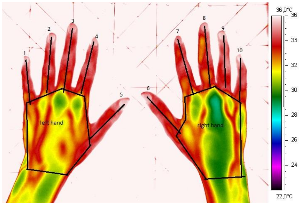
Fig. 9. The regions of interest (ROI's) measured on the fingers and the back of the hands. The temperature scale is shown on the right.
