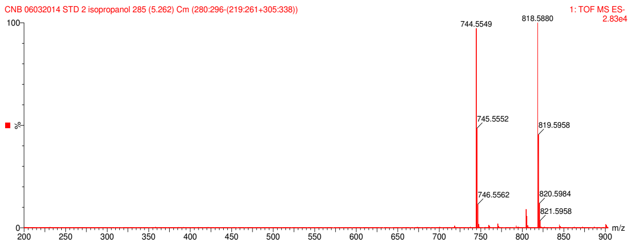
Appx. Figure 16: MS E full scan spectra recorded for 16:0-18:1 \Delta^9 PC upon CID. Analysed on Acquity UPLC BEH C18 column 50 mm using mobile phase gradient 3.
