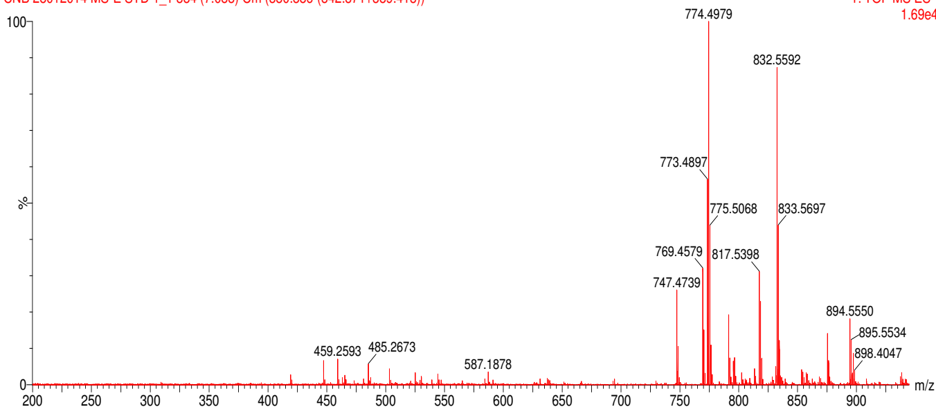
Appx. Figure 13: MS E full scan spectra recorded for 18:0-22:6 \Delta^{4,7,10,13,16,19} PC upon CID. Analysed on Acquity UPLC BEH C18 column 50 mm using mobile phase gradient 2.
