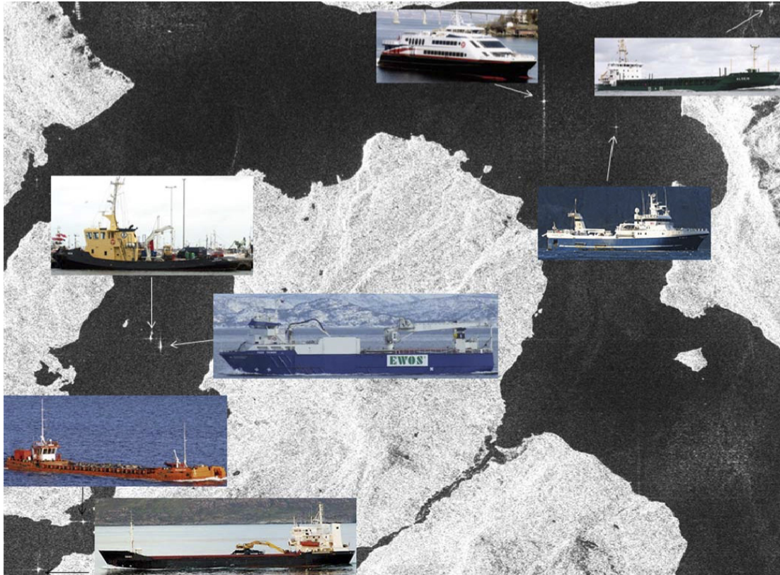
Figure 1.2: RADARSAT-2 Standard Quad-Pol SAR image in HH polarization acquired on 19 th September 2010. The image shows seven ships that are detected in the SAR image and confirmed by aisonline.com (from [10]).
