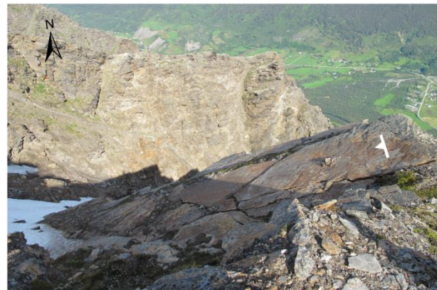
Fig. 25 Photo showing the eastern delimitation of the unstable area and exposed foliation surfaces striking NE with a gentle dip ( 30^\circ ) to NW. Photo by Böhme (NGU).
