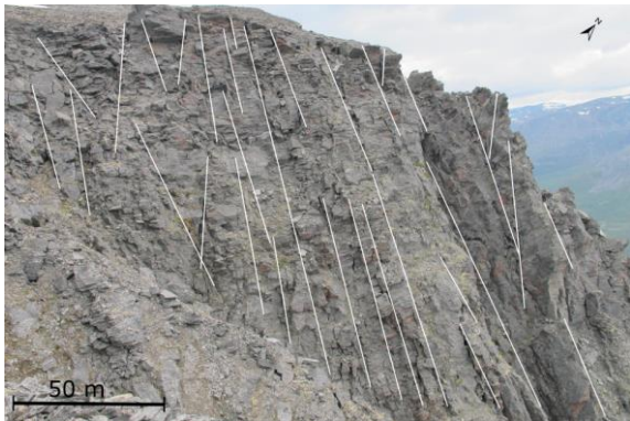
Fig. 26 Photo showing the western delimiting scarp in NNE-SSW cross-section view cut by back fracture scarp parallel fractures. Photo by Böhme (NGU).
