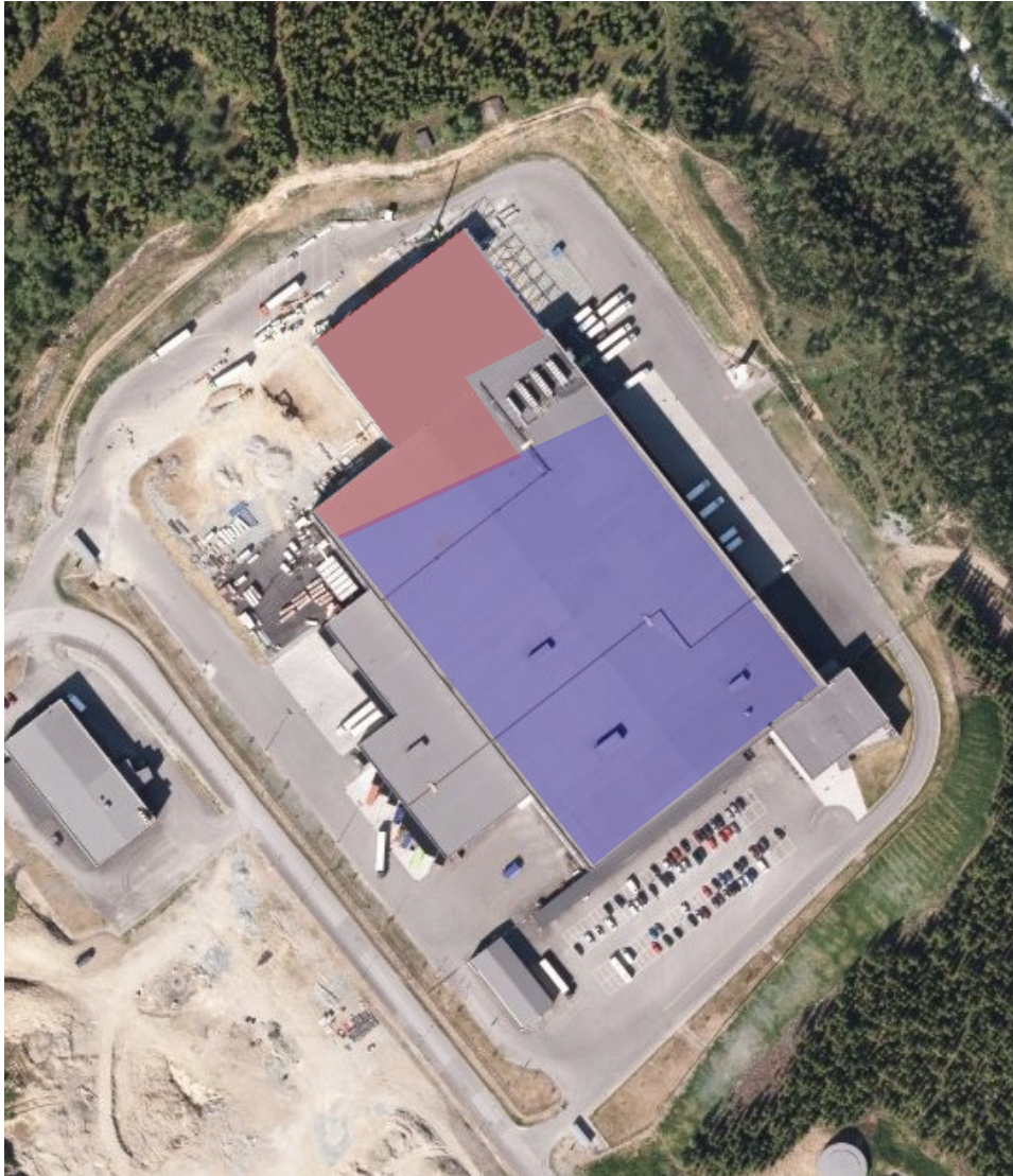
Figure 4.18: Aerial photo over Asko's. The blue section indicates the area where the majority of the turbulence is below twice the height of the building, and the red section indicates the area where the turbulence have a tendency to be above twice the height [photo from kartverket.no]
