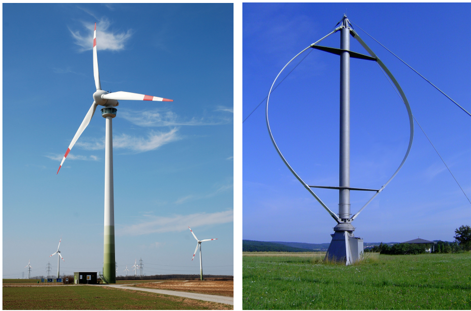
(a) Horizontal-axis wind turbine. Photo from [22]. (b) Vertical-axis wind turbine. Photo from [44].
