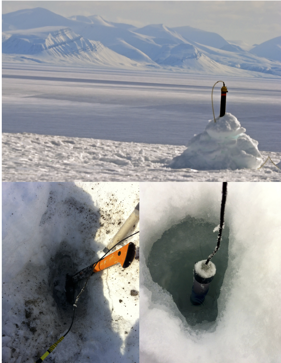
FIGURE 4.1: Induction coil magnetometer and electrode installations. (a) A coil installed to measure the H_z component. (b) Due to frozen surface and permafrost, often challenging to get a good contact to the ground. (c) An electrode being buried in an ice pool filled with a salty solution.
