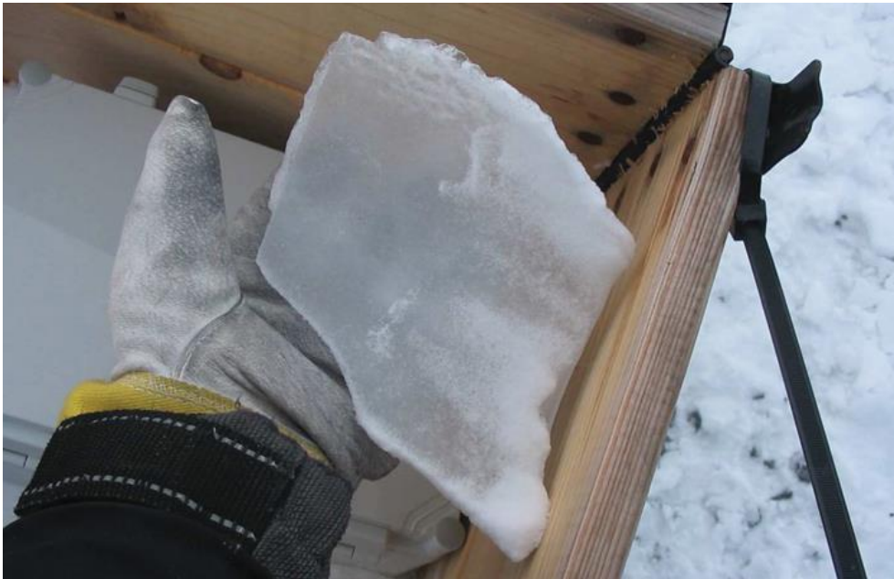
Figure 1: Piece of ice shed from a turbine in Nygårdsfjell wind park, Narvik, Norway [5]
