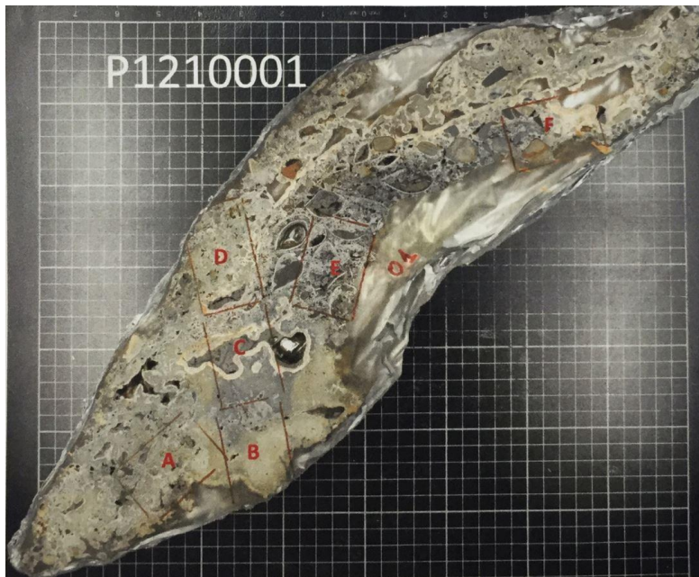
Fig 5.6: Overview image of the crust P1210001, the red rectangles indicates the location of the polished thin sections A-F. The smallest squares in the white grid lines indicates 1 cm * 1 cm.
