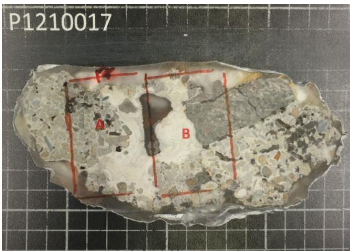
Fig 5.17: An overview of the crust P1210017, with the thin sections A-B indicated in the red rectangles.
