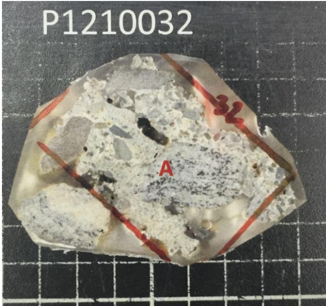
Fig 5.19: An overview of P1210032, one thin section made from the crust.
