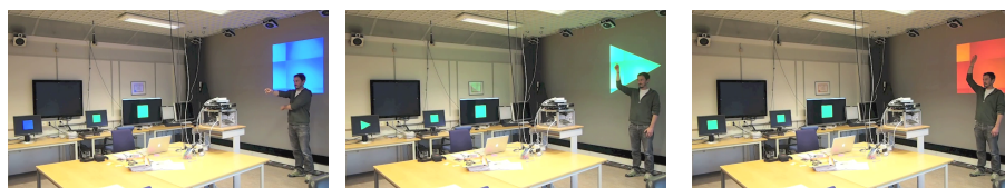
(a) Selection of computer across the room. (b) Action execution on the selected computers. (c) Single selection deselects the other computers.
