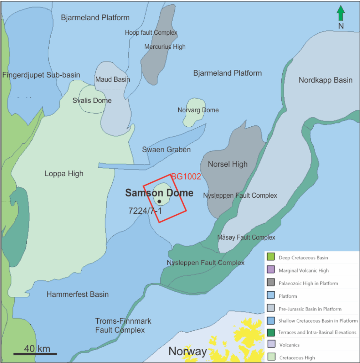
Figure 5-1. Location of the seismic dataset BG1002 (red rectangular) at Samson Dome, well 7224/7-1 (black dot) and main structural elements next to them. Modified from NPD FactMaps 2016.
