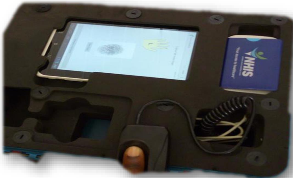
Figure 6: NHIS authentication device used for verifying patients visiting the health facility (Available at: https://twitter.com/nhis_ghana/status/682162762617884672 )
