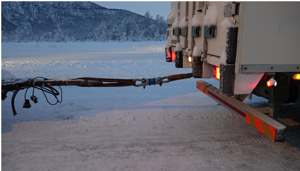
Figure E.2: Connection of the weight between the truck and the trailer.
