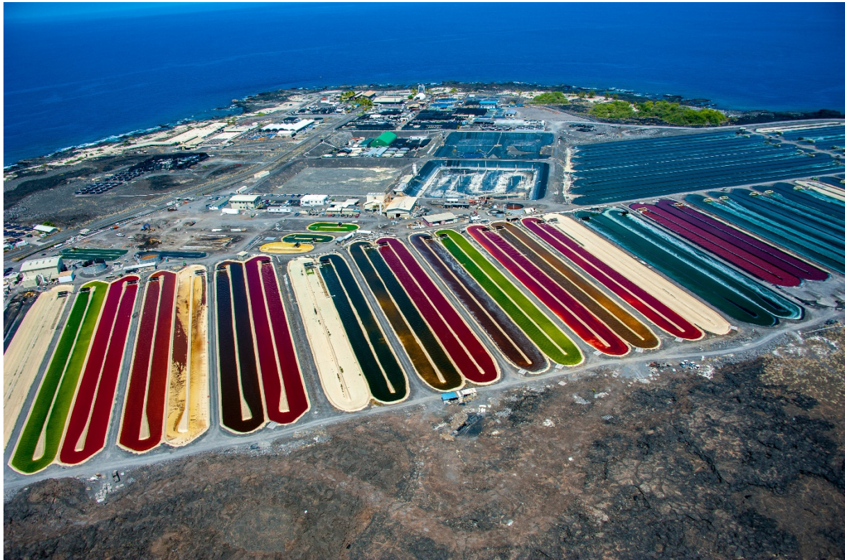
Figure 5 The open raceway ponds of Cyanotech, located in Hawaii. Picture used with permission, photo credit Cyanotech.
