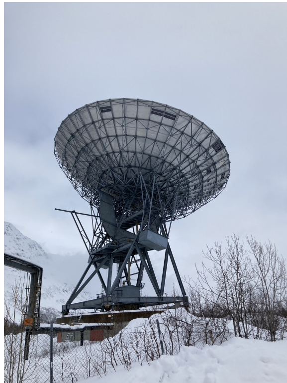
Figure 4.2: The EISCAT UHF radar at experiment day – 12/04/2021. In the image the radar is set to the appropriate pointing direction.
