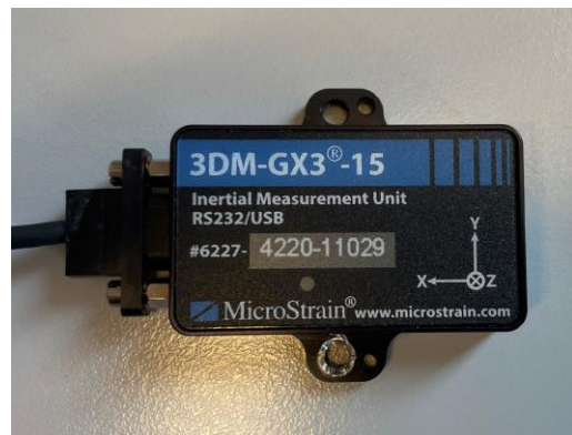
b) Microstrain MRU, model 3DM-GX-15 used on vessel model, Picture: Own archive.
