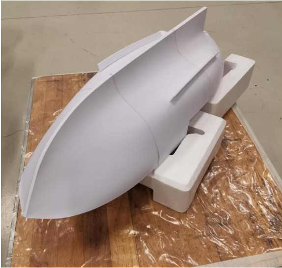
a) Before priming and coating, with bilge keel mounted.
