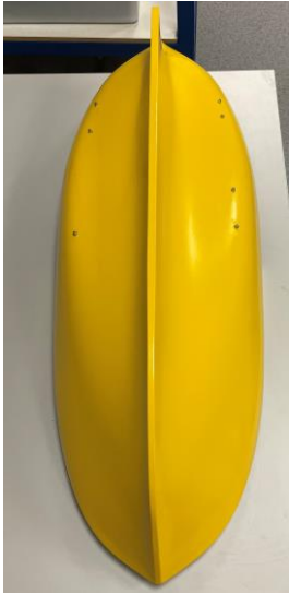
b) After priming and coating, without bilge keel mounted.
