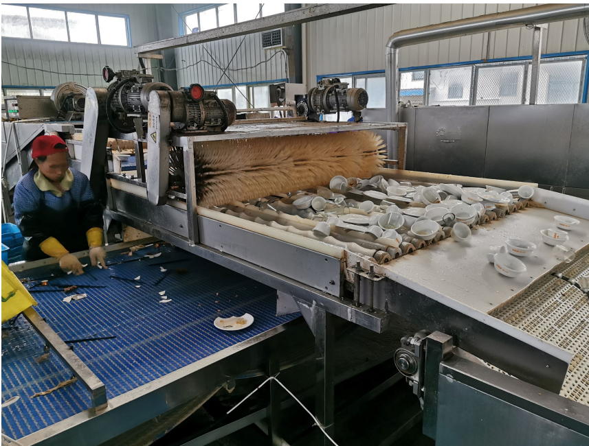
Figure 1.3: The sorting machine for tableware. Spoon and chopsticks as the smaller ones will fall to the lower conveyor belt from the gaps in the upper conveyor
