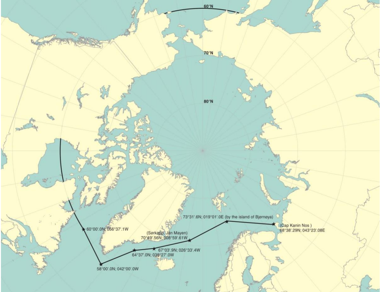
Figure 1 - Maximum extent of the Polar Code's Arctic waters application (IMO, 2017a, p. 9)
