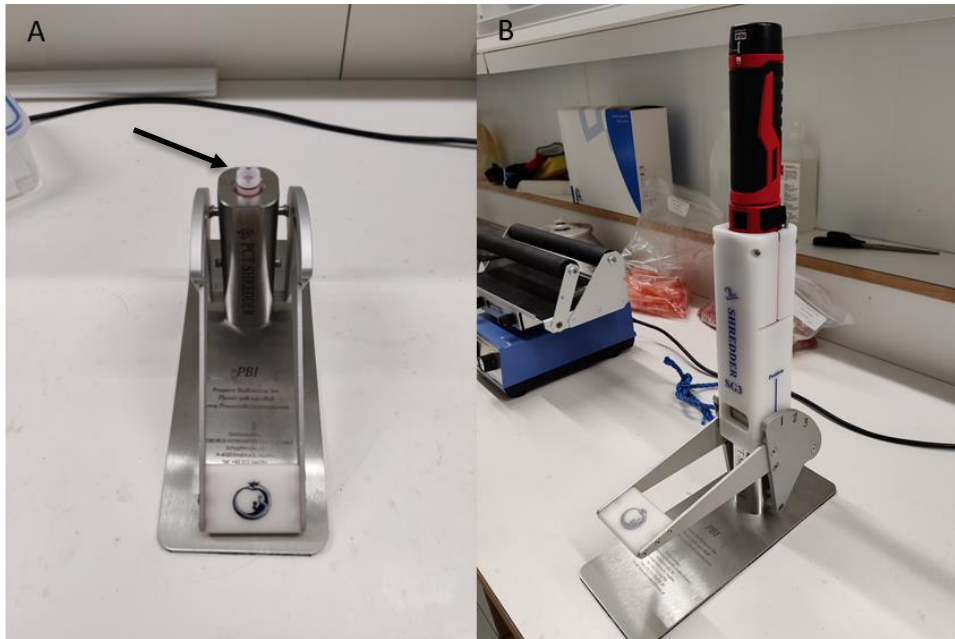
Figure 18. The shredder and cooling block provided by Oroboros instruments (Innsbruck, Austria). A: Shredder tube (indicated with arrow) inserted into the cooling block. B: The shredder inserted on the cooling block, set at position 1.
