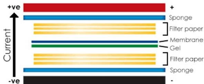
Figure 17. Orientation of Sponges, filter papers, the gel and membrane in a Western Blot transfer.
