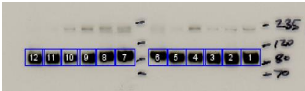
Appendix C Fig.3. 12 bands showing SERCA2a expression. Bands were highlighted using ImageJ software.
