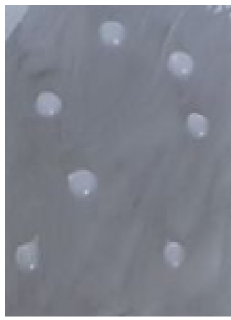
Figure 69: 10% of ZnSt, 10:1 PDMS to curing agent ratio.
