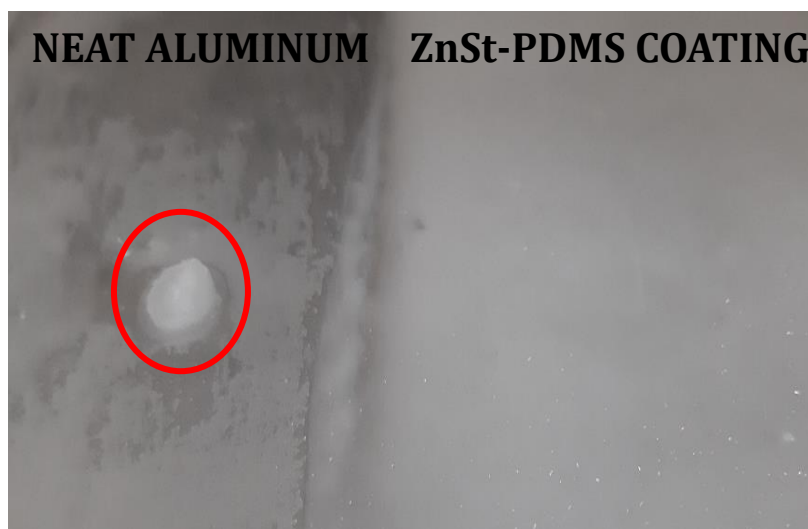
Figure 74: Ice adhesion between neat aluminum and ZnSt-PDMS coating.
