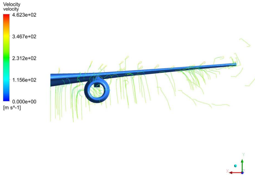
Figure 55: Velocity streamlines without glaze ice (front view).
