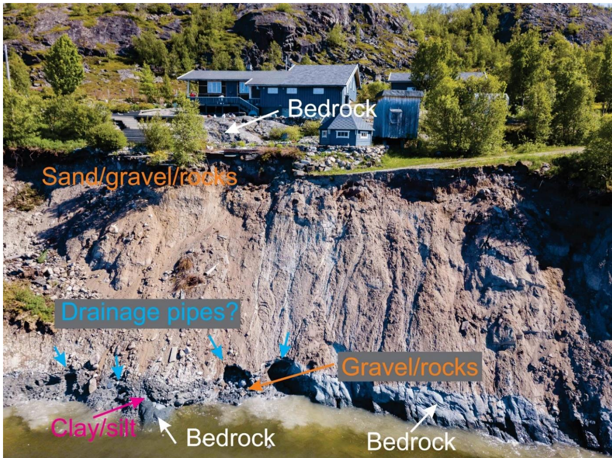
Figure 36: Photo of scarp three weeks after the landslide. Plumes of fine material indicate possible active drainage pipes, even two-three weeks. Photo: Raymond Eilertsen.
