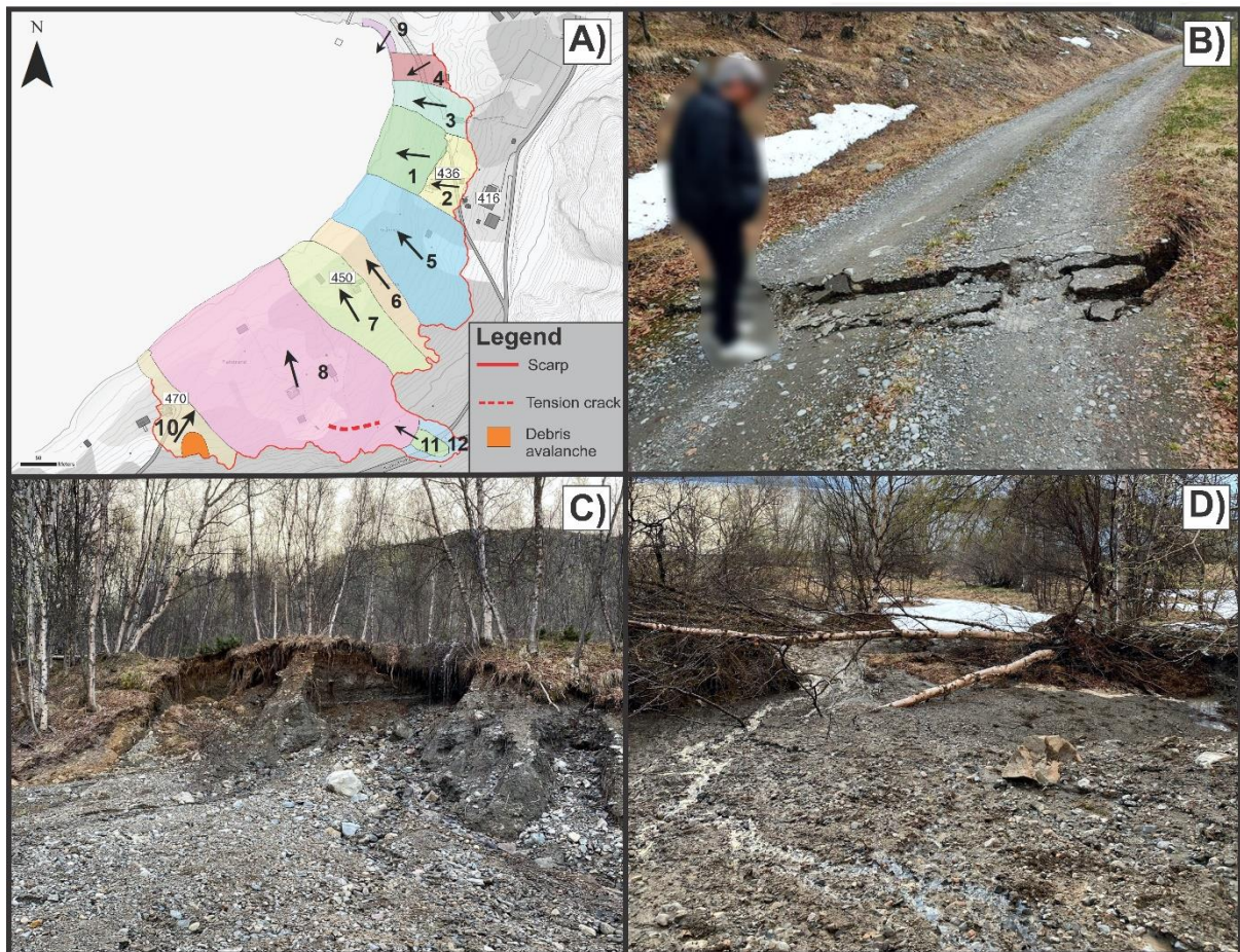
Figure 23: A) Overview map of Kråknes. B) Tension crack discovered on the 2nd of June (Photo: Jan Egil Bakkeby). C/D) Small landslide reported by locals on the 30th of May (Photo: Marit Ekerhovd).
