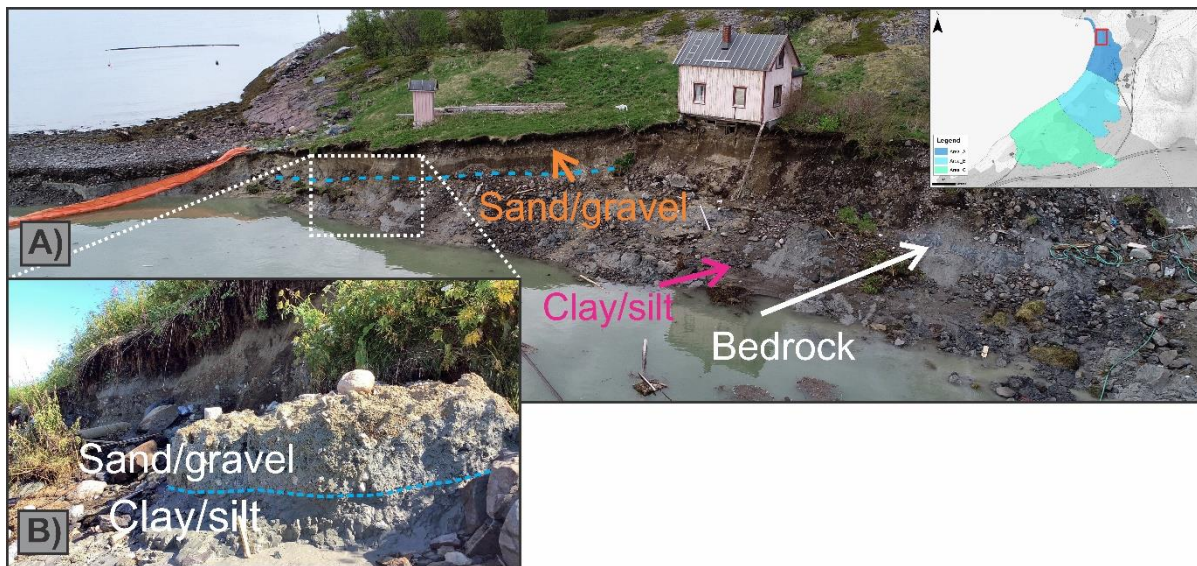
Figure 34: A) Photo taken in the NE direction. A layer of sand/gravel is observed above soft clay. Smaller areas of bedrock are exposed. B) Close-up photo of clay and sand/silt boundary (photos: Anders Bjordal, June 4th 2020).
