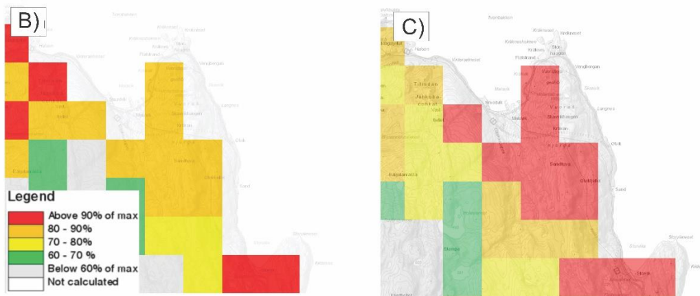
Figure 30: A) Graph of the groundwater level at Lakselv. The percentiles are based on the data from 1957-2020 (Xgeo.no). Yellow stars indicate the timing of the smaller debris avalanche, tension crack and sliding initiation. B) Groundwater volume in % of maximum for 27.05.2020 (source: xGeo.no, 1 km 2 grids). C) Groundwater volume in % of maximum for 03.06.2020 (source: xGeo.no, 1 km 2 grids).
