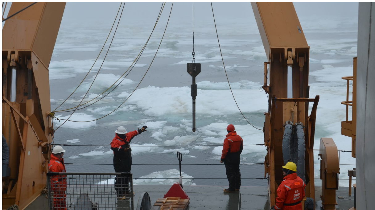
Figure 5. Gravity corer is used for coring soft sediments from the sub seabed. It weights two tons and consists of a six meters long steel core barrel with heavy lead weights (1600kg) on top. The steel core barrel houses an internal plastic core with inner diameter of 10 cm. The vessel is equipped with a winch and a long wire rope to lower the corer above the seafloor. Once allowed to freefall, the gravity corer relies on its weight and the gravitation to penetrate the seafloor. (Photo: https://www.usgs.gov/media/images/gravity-corer-recovers-uppermost-1-2-meters-sediment )
