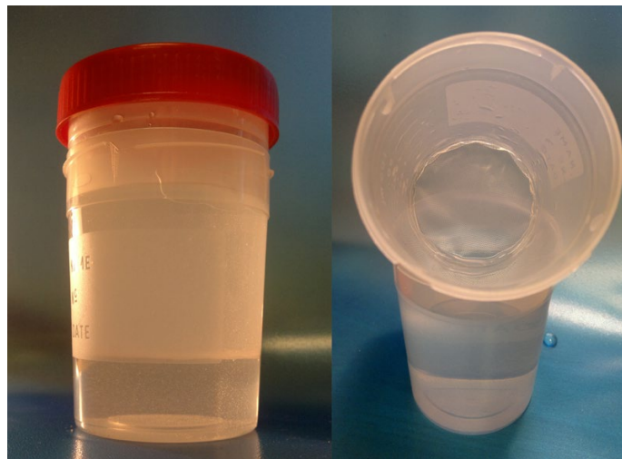
Figure 5: Egg production chambers used in experiments in Paper I and III. Left panel shows a vertical view of the two beakers stacked within each other with a lid on top. Right panel shows the inner cup lifted up showing the plankton netting used to separate the females from produced eggs and fecal pellets.
