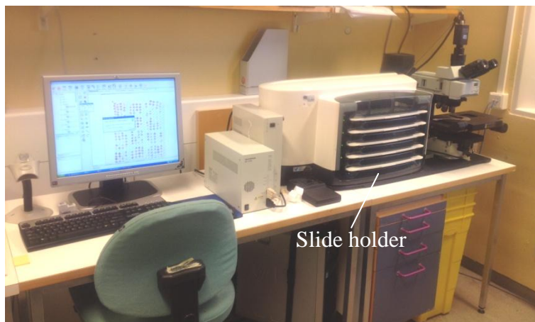
Figure 14. The Ariol imaging system provides digital imaging and scanning of IHC and ISH stained histological sections. The platform includes the software package, the computer screen, the slide holder, and the microscope [98]. The Ariol platform at IMB, UiT.
