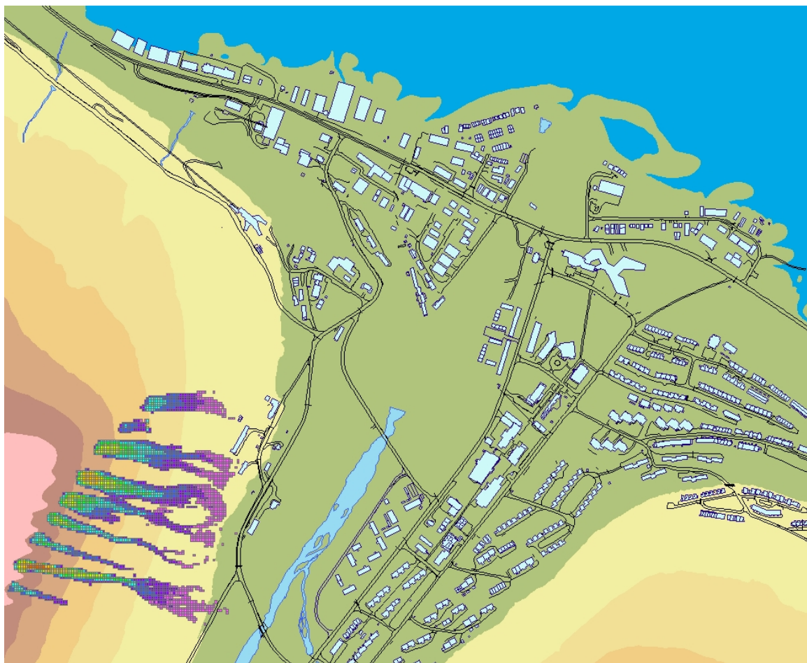
Figure 36: Maximal flow height of several possible debris flows at the northwestern outlet of Longyeardalen
